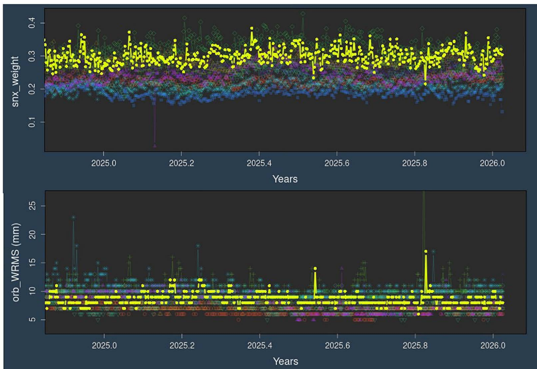
Figure 1: Sinex combination weight (top) and Orbit WRMS (bottom) with respect to IGS final solutions for the AC contributions, as computed by the IGS/ACC (GRG contribution highlighted in yellow). The corresponding plots are available via the IGS Plotter at https://igsac-cnes.cls.fr/html/links.html
