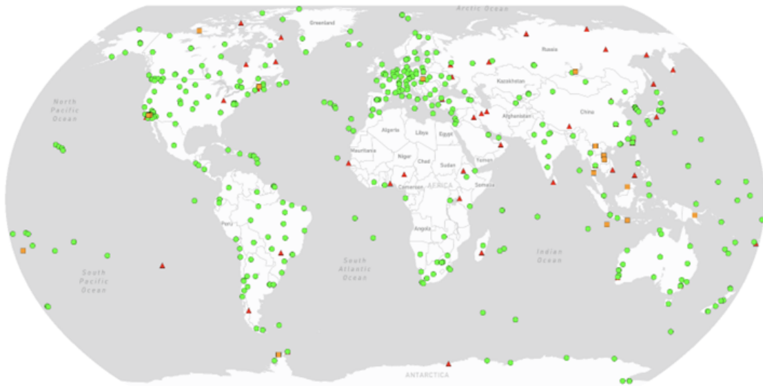
Figure 1: The IGS Network, as of the 1 st of January 2025. The map showcases 522 stations in total, including 388 tracking multiple GNSS constellations and 327 having real-time caster capabilities. The IGS collects, archives, and freely distributes Global Navigation Satellite System (GNSS) observation data sets from a cooperatively operated global network of ground tracking stations. The live version of this map is available at https://network.igs.org .
