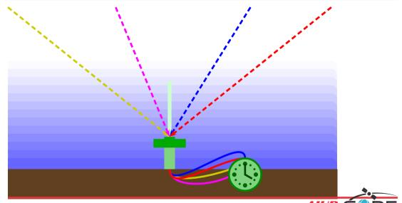
With GNSS-specific receiver clock corrections, the power of the multi-GNSS solution is significantly reduced (288+ additional parameters per station).
