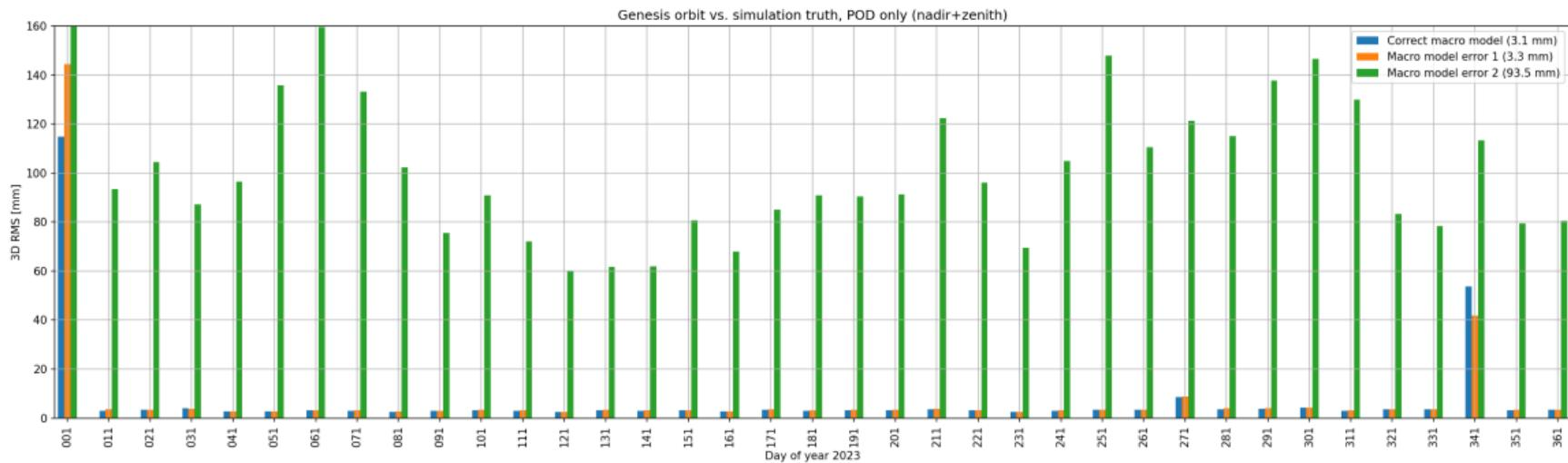
Significant degradation of Genesis orbit for macro model error 2 (solar panel front)
