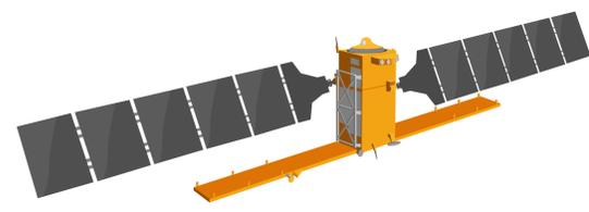
Figure 3: Sentinel-1 satellite with large SAR antenna on the bottom (image from <https://blogs.fu-berlin.de/reseda/sentinel-1/>). The SBF has its origin in the center on top, the  $x$ -axis points into the direction of the left solar panel axis (flight direction) and  $z$  down towards the SAR antenna. The right solar panel can cast a significant shadow onto the back side of the SAR antenna.
