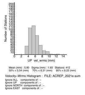
Figure 2: Histogram of the weighted root-mean-square (WRMS) scatter of daily position estimates of site used more than 5 times for 2021 after removal linear trends and elimination of gross outliers (5 times WRMS scatter). The median scatters are similar to last year with 1.6, 1.5 mm horizontal and 5.5 mm vertical.
