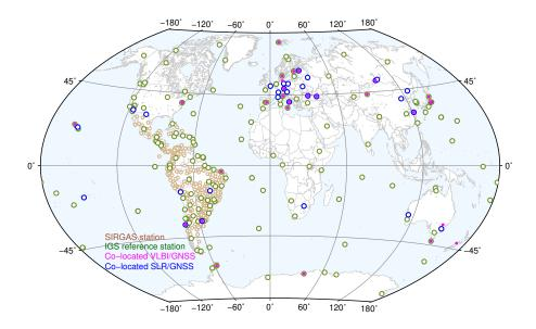
**Figure 5:** GNSS stations included in SIRGAS-Repro2. VLBI/GNSS (magenta dots) and SLR/GNSS (blue circles) co-located stations are foreseen for the combination of GNSS, SLR and VLBI normal equations. IGS core stations (green circles) are necessary for a high-quality GNSS data processing.
