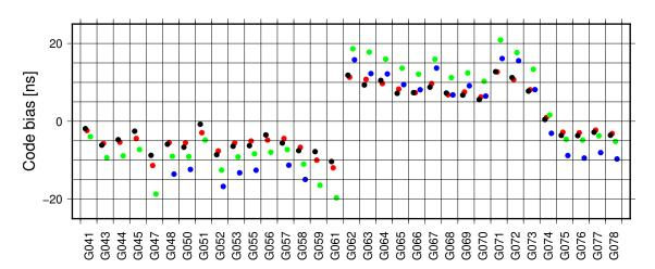
Figure 1: Observable-specific code bias (OSB) estimates for GPS code observable types (using the RINEX3 nomenclature) and GPS SV numbers, computed at CODE, for January 2022. Note that G043–G061 correspond to Block IIR, IIR-M; G062–G073 correspond to Block IIF satellite generations and G074–G078 corresponds to Block IIIA. Legend: C1C (black), C1W (red), C2W (green), C2L/C2S (blue).
