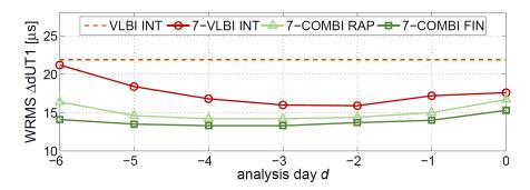
**Figure 5:** WRMS values of dUT1 estimates resulting from different analysis approaches compared to the IERS Bulletin A series. The analysis epoch is 12 h.
