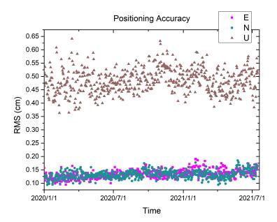
**Figure 4:** RMS errors (cm) of daily multi-GNSS PPP-AR positions in the east, north and up components at about 200 globally distributed stations against IGS weekly solutions after a Helmert transformation.
