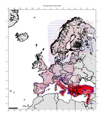
Figure 2: Strain rates derived from the data set of the EU Dense Velocities (using Dionysos Satellite Observatory StrainTool).
