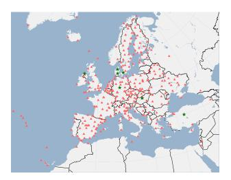
**Figure 1:** New GNSS stations (in green) integrated in the EPN in 2021. The new Norwegian station is not shown on the map.
