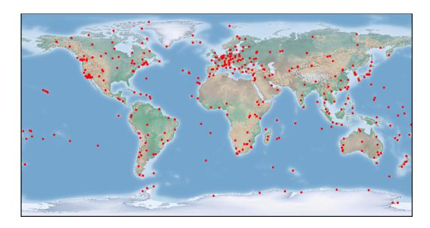
**Figure 2:** The 509 IGS stations as of January 31, 2021. The IGS collects, archives, and freely distributes Global Navigation Satellite System (GNSS) observation data sets from a cooperatively operated global network of ground tracking stations.
