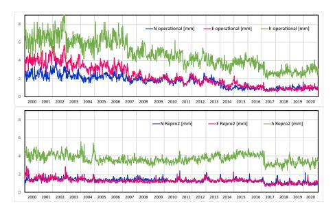
**Figure 3:** RMS values of the differences between the operational weekly SIRGAS solutions (transformed to IGS14/IGb14) and SIRGAS-Repro2 weekly coordinates with respect to the weekly coordinates of the IGS stations in IGS14/IGb14.
