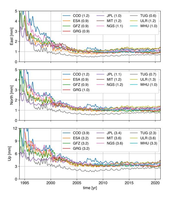
**Figure 3:** Median formal errors of station positions in daily re-weighted AC repro3 solutions. All time series were low-pass filtered with a 2.5 cpy cutoff frequency. The numbers in the legends are the medians of the time series of daily median formal errors for the period after 2005.0, in mm.
