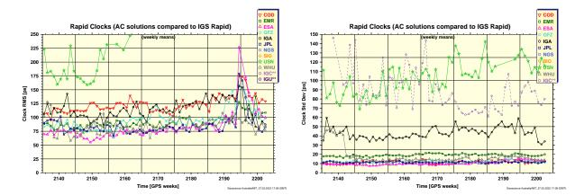
**Figure 5:** Weighted RMS (left) and standard deviation (right) of ACs Rapid clock submissions (smoothed). IGC\*\* are 24-hour products each containing four 6-hour segments from each update interval of the IGS real-time stream. IGU\*\* consists of four separate comparisons to IGR done each day over the first 6 hours of each IGS Ultra-rapid product.
