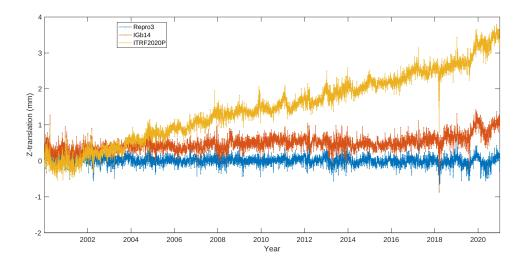
**Figure 8:** Similar to Figure 2 but for the Z-component. The Repro3, IGb14 and ITRF2020P rates are -0.00, 0.02 and 0.15 mm/yr, respectively.
