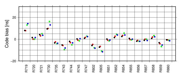
**Figure 2:** Observable-specific code bias (OSB) estimates for GLONASS code observable types (using the RINEX3 nomenclature) and GLONASS SV numbers, computed at CODE, for January 2022. Note that R719–R747 and R851–R860 correspond to GLONASS-M; R802–R805 correspond to GLONASS-K1 satellite generations. Legend: C1C (black), C1P (red), C2P (green), C2C (blue).
