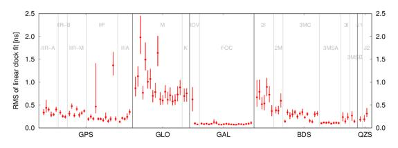
**Figure 4:** Boxplot from the RMS of a linear fit of the satellite clocks during 24 hours obtained from the MGEX solution of the year 2021.
