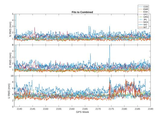
Figure 3: RMS scatters of the fits of the different IGS ACs to the MIG combined solution for 2021. The increase in scatter between wees 2175 and 2186 is due to due -180 mm height errors at DRAO in the NGS AC results after the change from an TRM59800.00 antenna to an TWIVC6050 antenna at DRAO on 2021/09/03. After week 2186, the NGS DRAO result was removed from the combination.
