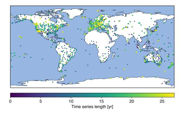
**Figure 2:** repro3 station newtork. The sizes and colors of the dots indicate the lengths of the repro3 combined position time series.
