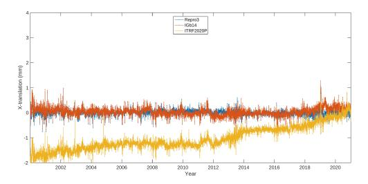
**Figure 6:** X translation estimates in aligning the MIT position time series to Repro3 (blue), IGb14 (brown) and ITRF2020P (dark yellow). The rates for the three reference frames are -0.00, 0.00 and 0.07 mm/yr, respectively, with zero rate with respect to Repro3 expected.
