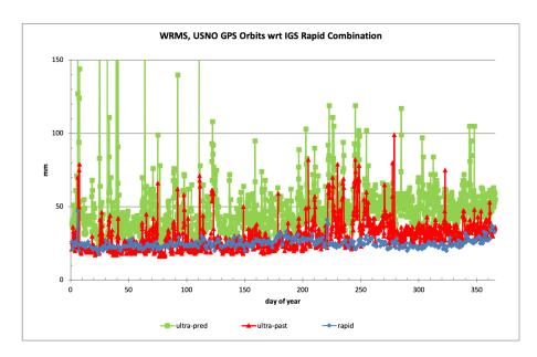
**Figure 1:** Weighted RMS of USNO GPS orbit estimates with respect to IGS Rapid Combination, 2021. "Ultra-past" refers to 24-hour post-processed section of USNO Ultra-rapid orbits. "Ultra-pred" refers to first six hours of Ultra-rapid orbit prediction.
