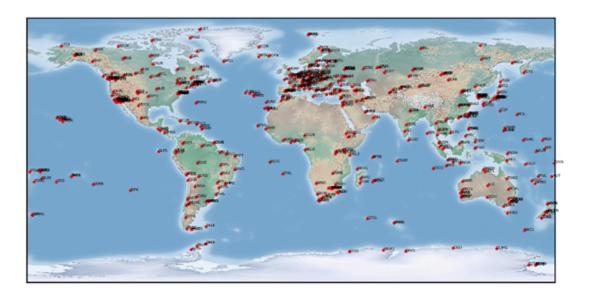
**Figure 1:** The 509 IGS stations as of January 31, 2021. The IGS collects, archives, and freely distributes Global Navigation Satellite System (GNSS) observation data sets from a cooperatively operated global network of ground tracking stations.
