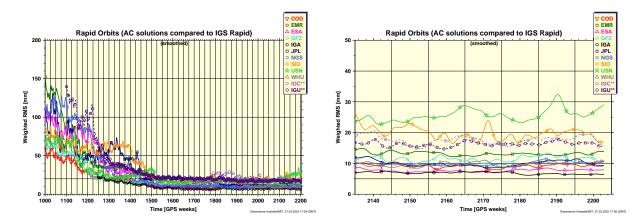
**Figure 4:** Weighted RMS of ACs Rapid orbit submissions (smoothed). The historical time series of comparison results is shown on the left, and recent comparison results are shown on the right. IGC\*\* are 24-hour products each containing four 6-hour segments from each update interval of the IGS real-time stream. IGU\*\* consists of four separate comparisons to IGR done each day over the first 6 hours of each IGS Ultra-rapid product.
