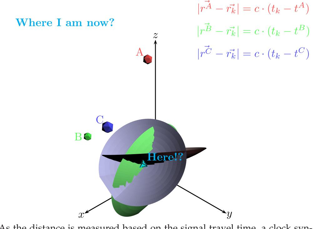
As the distance is measured based on the signal travel time, a clock synchronization between the satellite and receiver clock is necessary. Typically this is done by computing the related clock correction with respect to GPS-system time.
