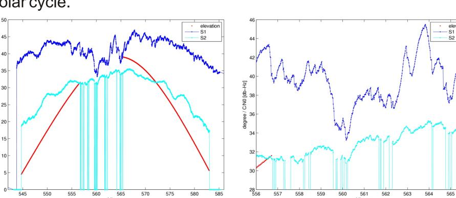
A typical image of the C/N0 values is shown in case of missing L2 observations (C/N0 (L2)= 0) in the middle of a satellite pass. The elevation shows that the missing observations occur near the highest elevation of the satellite pass. The different behavior of the C/N0 values as well as the different noise on the two frequencies are not yet understood and need further investigations.
