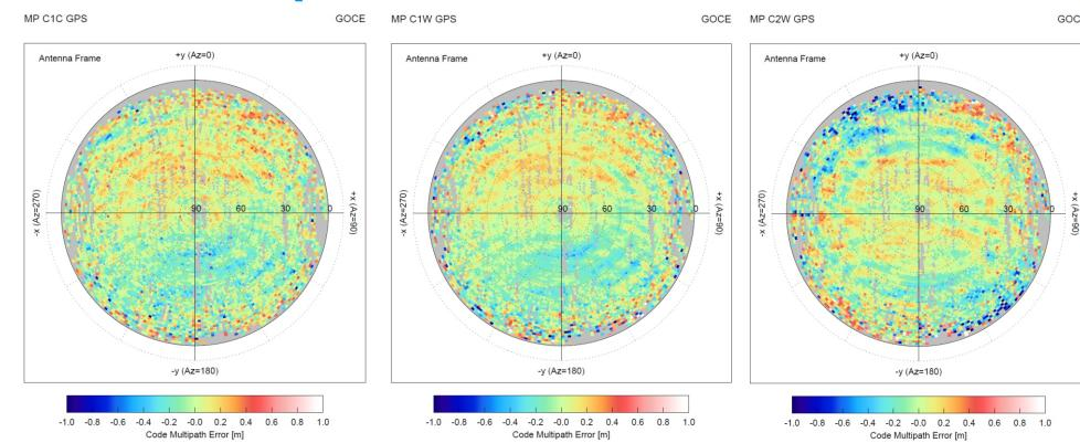
Code multipath errors for L1 C/A (left), L1 P(Y) (center) and L2 P(Y) tracking (right). The plots indicate the presence of moderate (<0.5 m peak error) multipath errors which are presumably caused by diffraction in the near-field of the antenna. For L1, a notable forward/backward asymmetry can, furthermore, be recognized, which might introduce systematic along-track positioning errors in codebased orbit determination.
