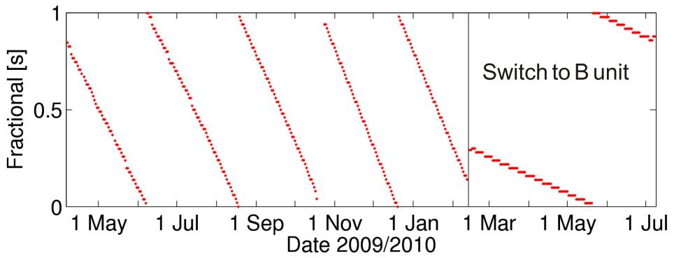
The internal clock is not steered to integer seconds and the observation epochs have, therefore, fractional offsets (shown at the midnight epochs). These fractional offsets stayed constant for about 25-27h and then jumped by 20ms. This behaviour changed after the switch to the redundant onboard computer B mid of Feb 2010. The time interval for a constant fractional offset is extended to 5-6 days.
