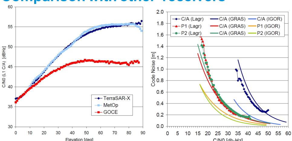
**Left:** A comparison of L1 C/N0 values for the TerraSAR-X (IGOR receiver), MetOp (GRAS instrument) and GOCE (Lagrange receiver) indicates a notably lower L1 gain of the helix antenna on GOCE as compared to the antennas employed on the other missions.
