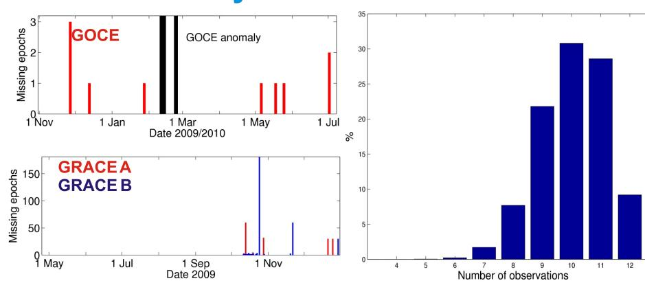
**Left,** top:The GOCE 1 Hz GPS data are almost continuous and only very few observation epochs are missing (1 bar/day). Bottom: Missing epochs (10 s !!) for GRACE A / B. **Right:** The percentages of the number of tracked satellites per epoch are shown for a typical day (November 6, 2009). For two thirds of the epochs ten or more observations are available.
