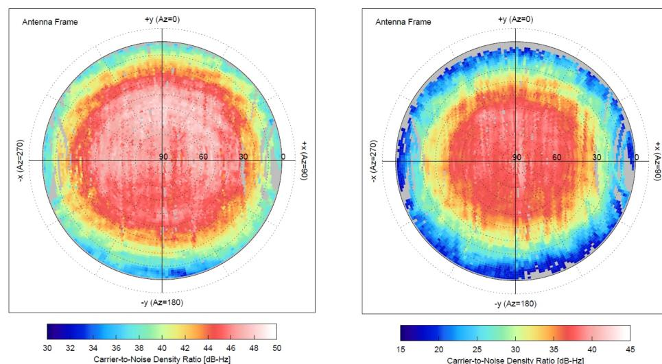
The variation of the carrier-to-noise-density-ratio (C/N0) for L1 C/A code tracking (**left**) and L2 P(Y)-code tracking (**right**) as a function of azimuth and elevation in the antenna diagram indicates a slightly higher L1 antenna gain in the forward direction. The flight direction corresponds to  $Az=0^{\circ}$ .
