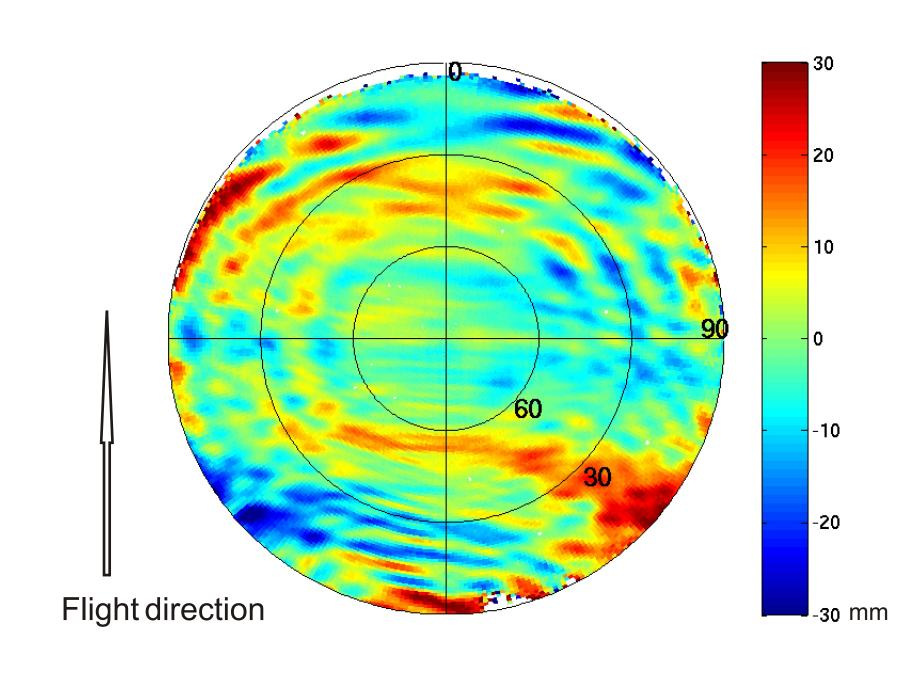
The empirically derived phase center variations (PCVs) of the main SSTI antenna show systematics up to several cm's. The carrier phase observations have to be corrected for the PCVs in the PSO (Precise Science Orbit) processing to achieve the required orbit accuracy.
