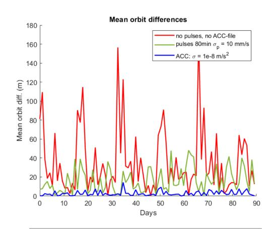
Average orbit distance between the simulated reference orbit, and the final estimated orbit for each 25h arcs.
