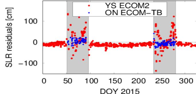
Significant reduction of SLR residuals and CLK-fit RMS during ON-periods (QZS-1, 3-day long arc solution)
