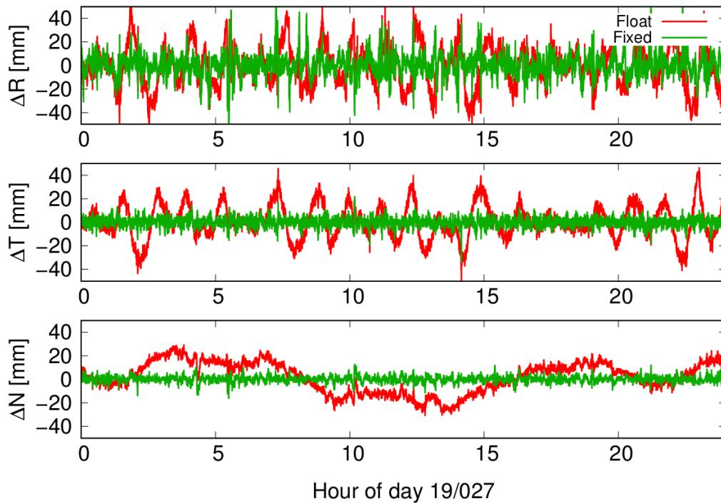
Example: Differences between reduced-dynamic and kinematic Sentinel-3A orbits for one day in radial, tangential and normal direction (ambiguity浮 and ambiguity固定)
