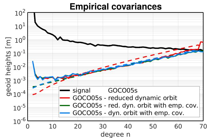
Dynamic orbit parametrisation features imperfect force model → solution degraded
