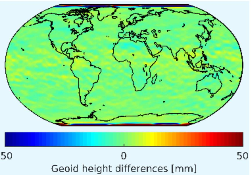
Geoid height differences of GPS-only solution for November 2009–July 2012 w.r.t. ITG–GRACE2016, 300km Gauss filter applied.
