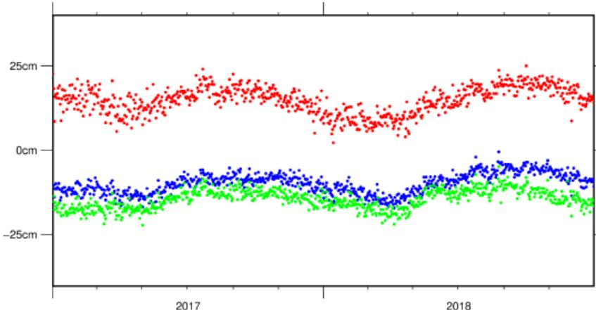
(a) Chamber calibrations: Scale fixed to ITRF 2014.
