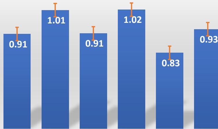
GRACE A, solar radiation pressure mean scaling factor over 3 months
