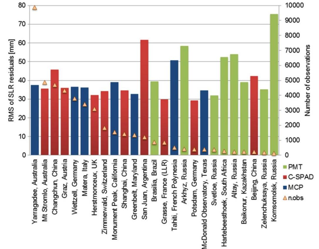
**Fig. 8** RMS of SLR residuals and the number of observations to Galileo collected by different SLR stations
