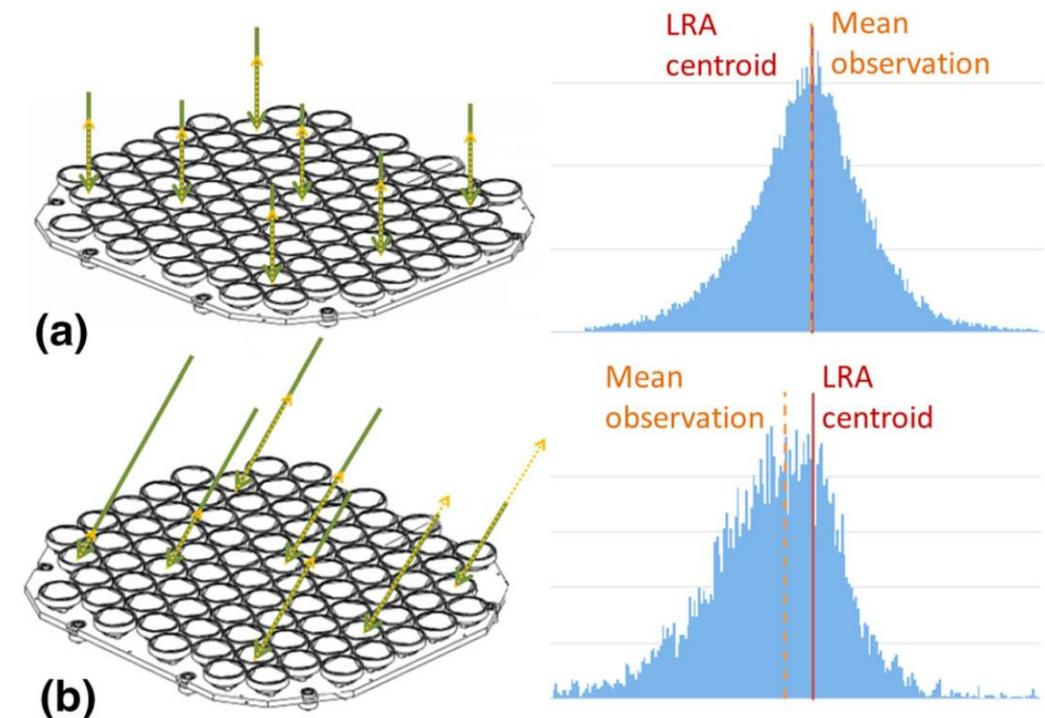
**Fig. 7** Satellite signature effect for multi-photon detectors: **a** the nadir angle is 0 and the LRA centroid coincides with the mean observation, **b** the LRA is inclined and the detection timing is defined at some threshold level at the leading edge of the return pulse; as a result, the mean registered range is shorter than the actual one
