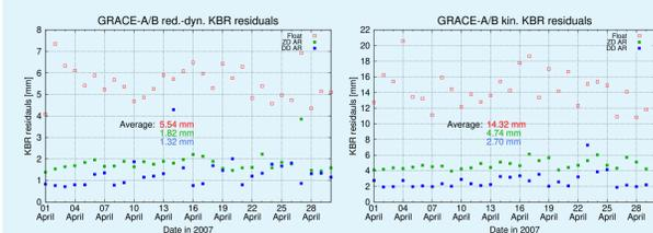
Figure 5: Daily RMS values of K-band residuals for reduced-dynamic (left) and kinematic (right) orbit and baseline solutions. For the kinematic solution statistics an outlier threshold of 10 cm was applied.
