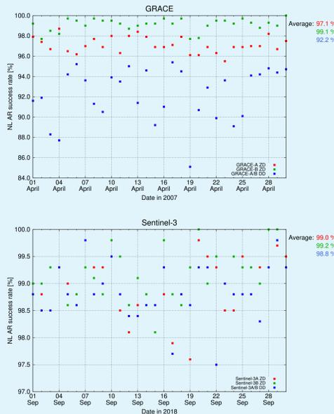
Figure 3: Percentage of resolved narrowlane ambiguities for GRACE (top) and Sentinel-3 (bottom). Red: ZD AR for LEO A. Green: ZD AR for LEO B. Blue: DD AR for baseline.
