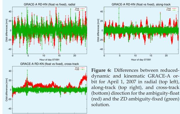
Figure 6: Differences between reduced-dynamic and kinematic GRACE-A orbit for April 1, 2007 in radial (top left), along-track (top right), and cross-track (bottom) direction for the ambiguity-float (red) and the ZD ambiguity-fixed (green) solution.
