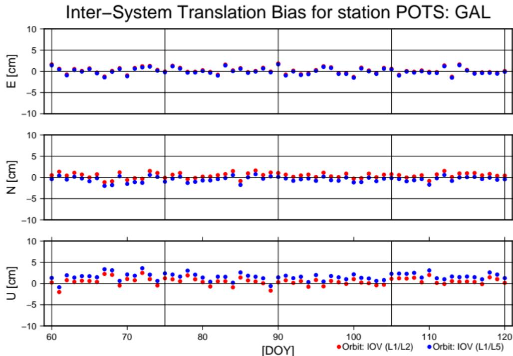
Figure: Galileo Inter-system translation bias: Station POTS
