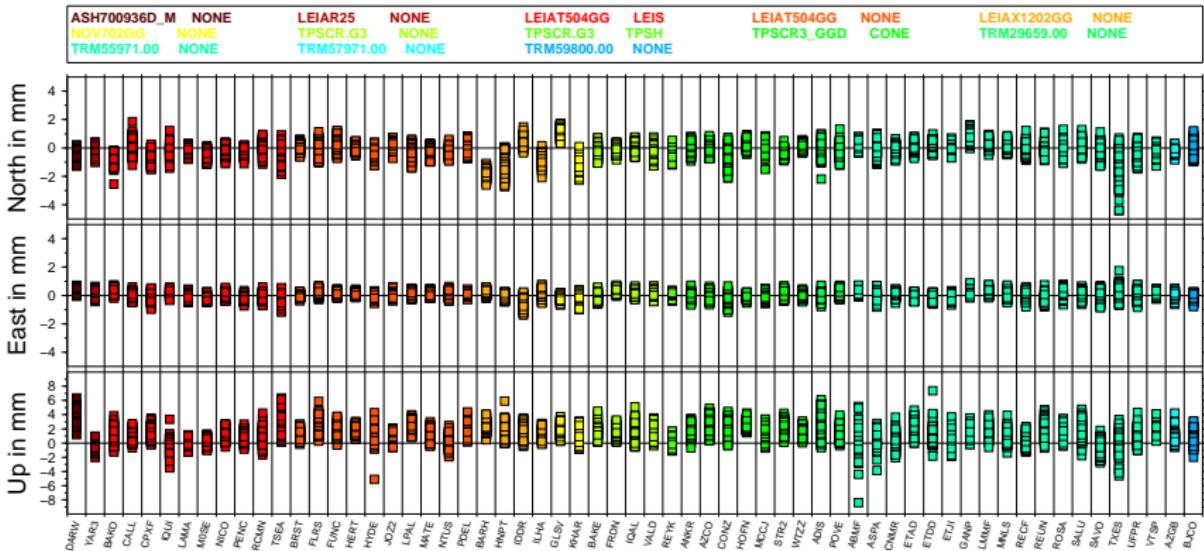
GPS–GLONASS–Bias for the coordinates using IGS05.atx–antenna phase center corrections from weekly solutions of the years 2009 and 2010.
