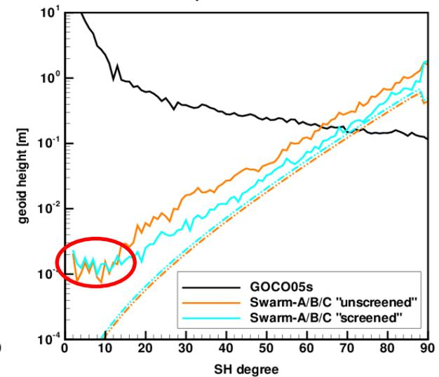
Impact of screening the raw RINEX GPS data files (dL4/dt criterion):
