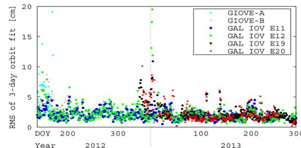
Fig. 4: RMS of 3-day longarc fit of CODE MGEX orbits (individual Galileo satellites).
