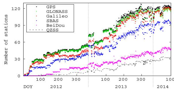
Fig. 1: Number of tracking stations providing data in RINEX3 format and considered in CODE's data monitoring.
