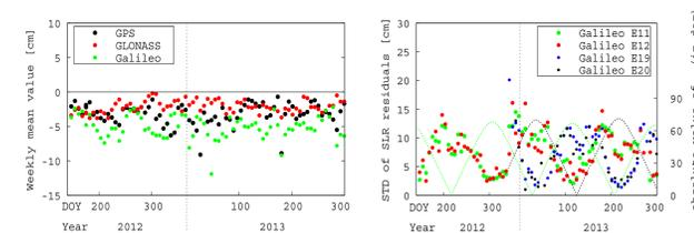
Fig. 5: SLR validation of CODE MGEX orbits. Left: Weekly mean offset of SLR residuals of GPS (G06, G30), GLONASS, and Galileo satellites (system-wise). Right: Weekly standard deviation of SLR residuals of individual Galileo satellites. The dotted curves show the absolute value of the Sun's elevation above the orbital planes ( $\beta$ ) of E11 and E12 (green), and E19 and E20 (black).
