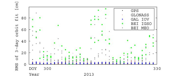
Fig. 7: RMS of 3-day longarc fit of CODE MGEX orbits (GPS, GLONASS, Galileo, BeiDou) for the time interval DOY 13/300 - 13/330.
