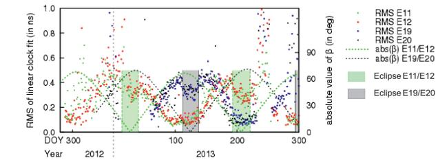
Fig. 6: Linear fit of CODE MGEX epoch-wise satellite clock corrections. Top: Galileo IOV. Bottom: GPS G01 and G25 (Block IIF). The dotted curves show the absolute value of the Sun's elevation above the satellites' orbital planes. The shaded rectangles mark the eclipsing seasons of the satellites. The large clockfit RMS for the Galileo satellites after DOY 13/230 is due to the switch from Maser to Rubidium clocks on all Galileo satellites.
