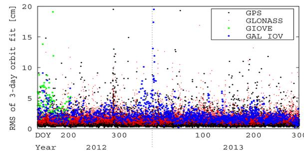
Fig. 3: RMS of 3-day longarc fit of CODE MGEX orbits (GPS, GLONASS, Galileo).
