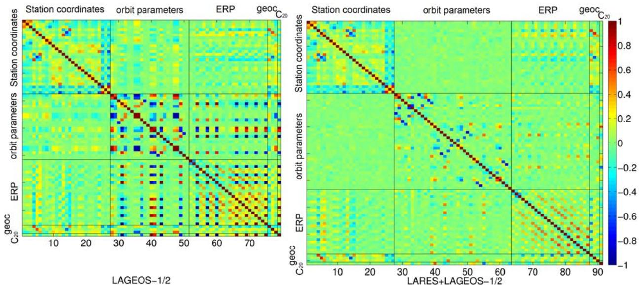
**Figure 3.** Correlation matrices of LAGEOS-1/2 (left) and LARES+LAGEOS-1/2 (right) for a 7-day solution. The matrices contain the core station coordinates, satellites orbits, Earth rotation parameters (ERP), geocenter coordinates, and  $C_{20}$ . All remaining parameters were pre-eliminated (range biases, pseudo-stochastic pulses, non-core station coordinates).
