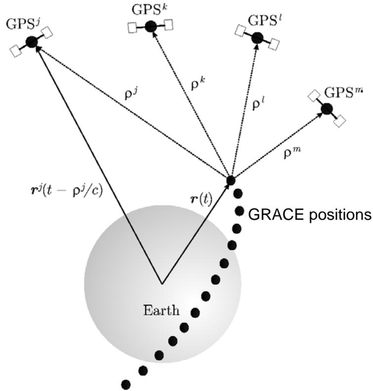
The GRACE satellites may be geo-located with cm-accuracy at any time, e.g., by a kinematic precise point positioning (PPP).
