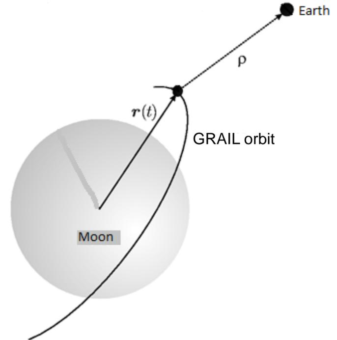
The orbits of the GRAIL satellites may be constrained by Doppler measurements from the Earth only on the near-side of the Moon.
