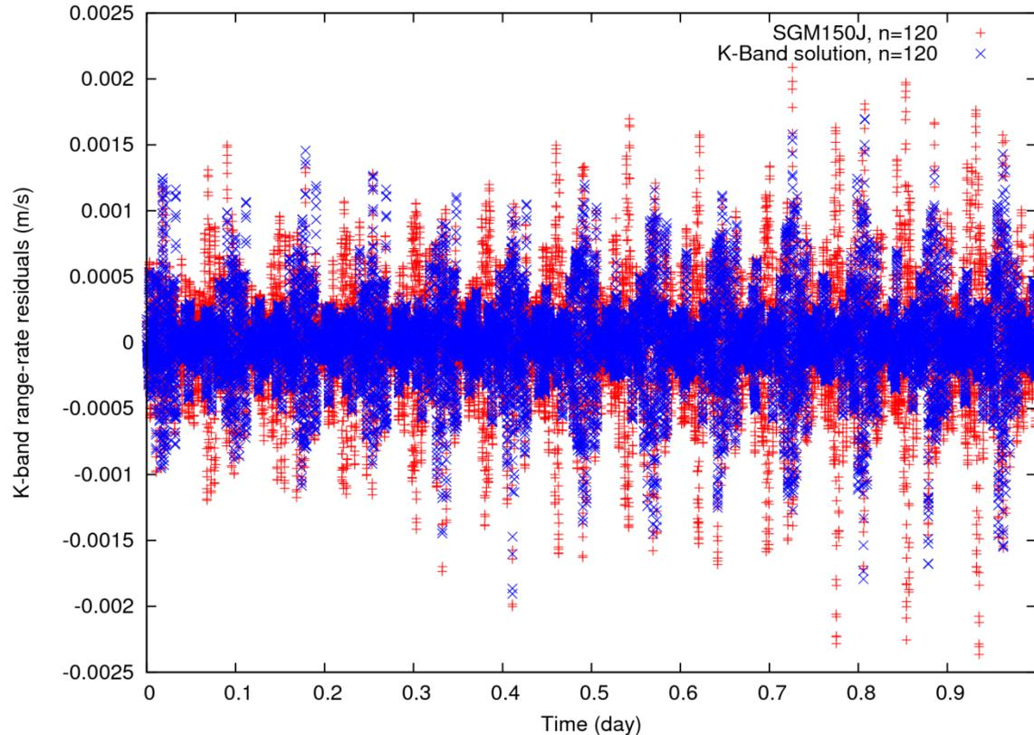
K-Band residuals of the [combined gravity field solution](#). An improvement with respect to the [SELENE solution](#) can be seen, but the residuals still contain a lot of systematic signal ...
