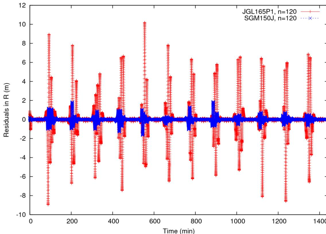
Radial position residuals for GRAIL-A from an orbit determination using position pseudo-observations. The **Lunar Prospector** and **SELENE** gravity field models up to  $n_{\max} = 120$  were used. Larger residuals on the far-side are clearly visible for both a priori gravity field models.
