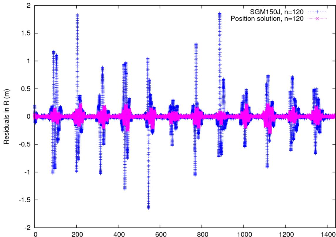
Radial position residuals for GRAIL-A from an orbit determination using position pseudo-observations. The **SELENE** and an **AIUB model based on positions** up to  $n_{\max} = 120$  were used. Residuals on the far-side are further reduced, but are still larger than on the near-side.
