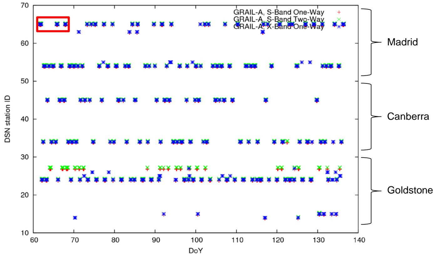
Radio-tracking of GRAIL-A by NASA's Deep Space Network (DSN) during the primary mission phase. Several of the 34-m antennas of the each complex of the DSN network have been used for tracking. The [X-Band One-Way](#) data are primarily used for orbit determination.
