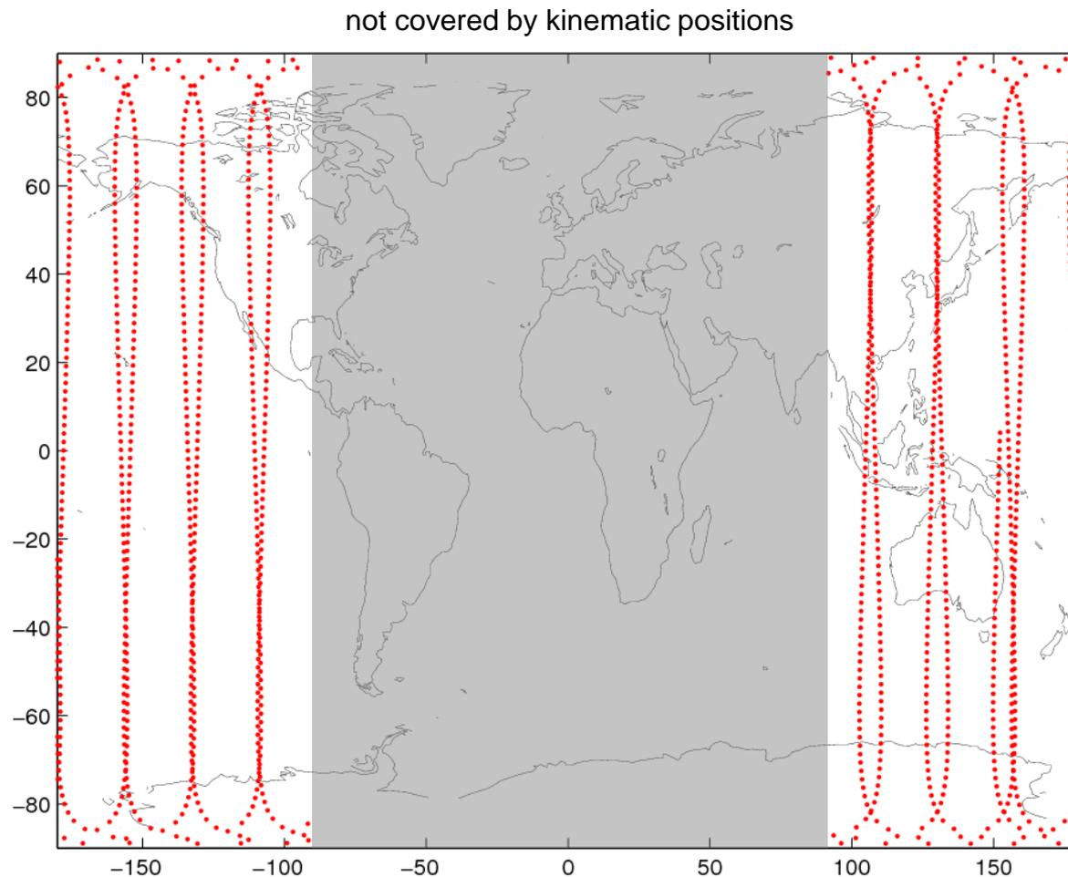
An artificial degradation of the coverage with kinematic positions is used in the following to illustrate the impact of a “far-side effect” for  $-90^\circ < \lambda < 90^\circ$  on the combined orbit and gravity field determination, whereas the K-Band observations are continuously available.
