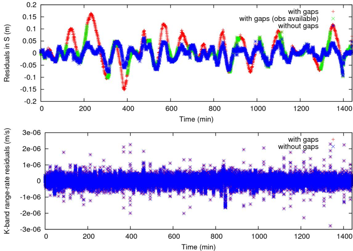
Along-track position residuals for GRACE-A from a combined orbit determination using K-Band and position pseudo-observations **with gaps** and **without gaps**. The AIUB-GRACE03S static gravity field model up to  $n_{\max} = 160$  was used, but **no** accelerometer data was used. Larger differences are now seen in the positions, but not in the K-Band residuals.
