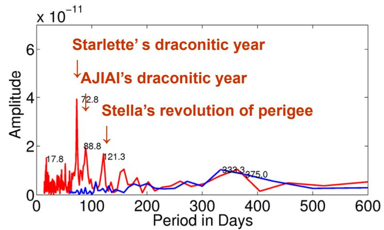
$C_{41}$  derived by SLR shows similar secular trend to the GRACE results, but the high-frequency part is affected by correlations and modeling deficiencies
