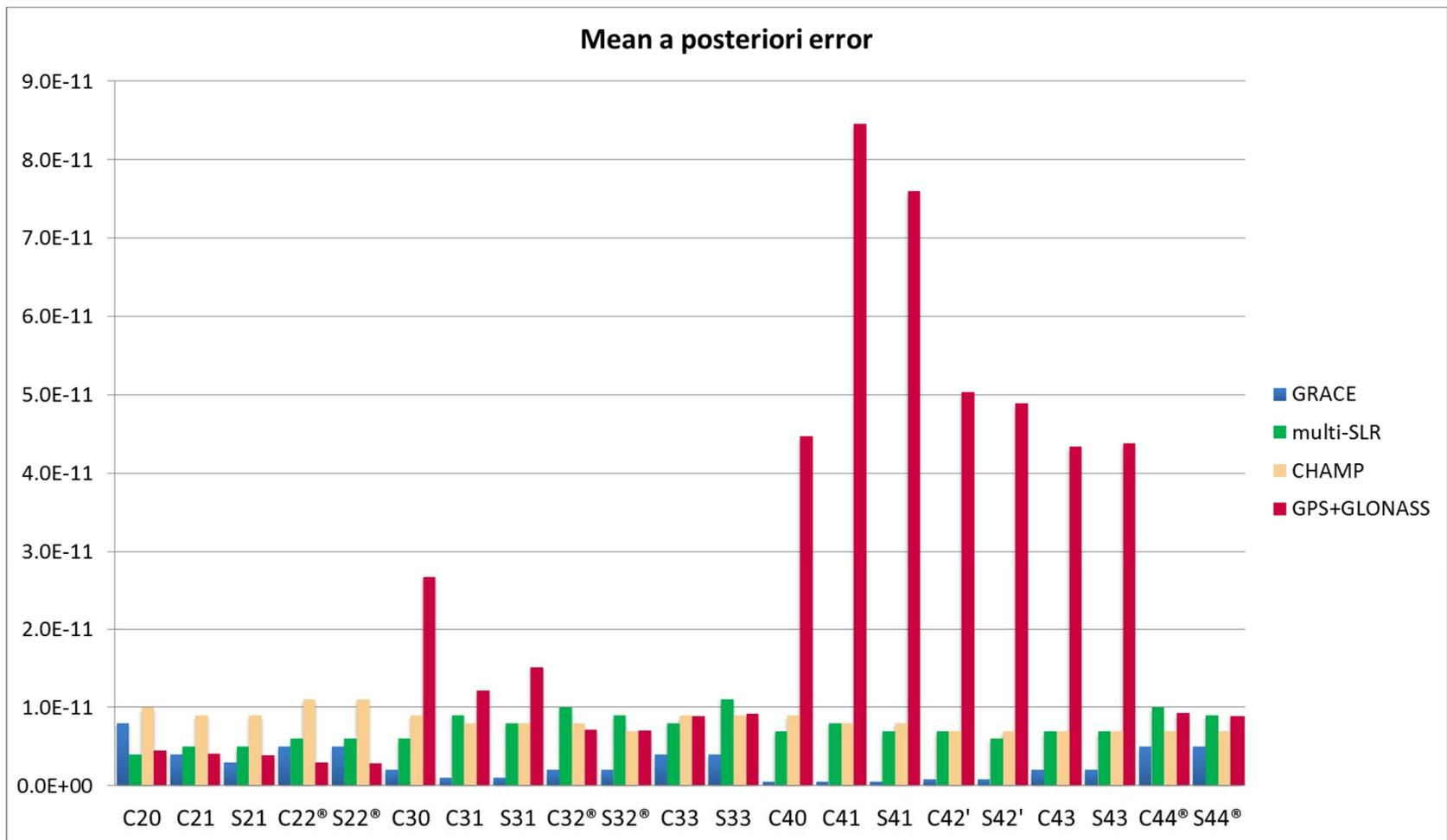
**GNSS** satellites are very sensitive to gravity field coefficients of degree 2. For coefficients above degree 3, GNSS are only sensitive to **resonant gravity field parameters** (®).
