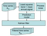
coefficients. The prediction model for the Kalman filter is derived by a least-squares adjustment from the original time series. A random walk is introduced as process noise allowing for variations w.r.t. the prediction model. The filtering is repeatedly applied with different instances of the process noise (ensemble Kalman approach) and solutions are averaged.
