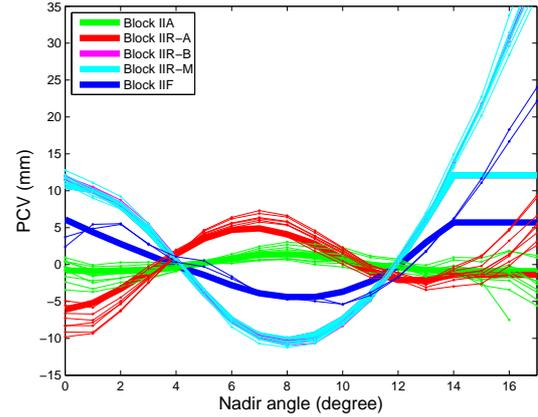
Figure 6. Estimated satellite-specific PCVs using LEO data (thin lines) and igs08.atx block-specific values used before the PCV extension beyond nadir angles of  $14^\circ$  (bold lines).
