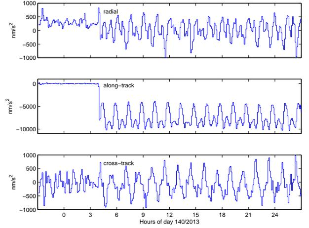
Figure 1. Piecewise constant accelerations estimated for GOCE on 20 May, 2013. Note the transition into non-drag-free flight and the different scale for the along-track component.
