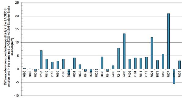
Figure 8. Difference of the repeatability of SLR station coordinates in the combined solution and in the LAGEOS-1/2 solution. Positive values denote a better repeatability in the combined solution.
