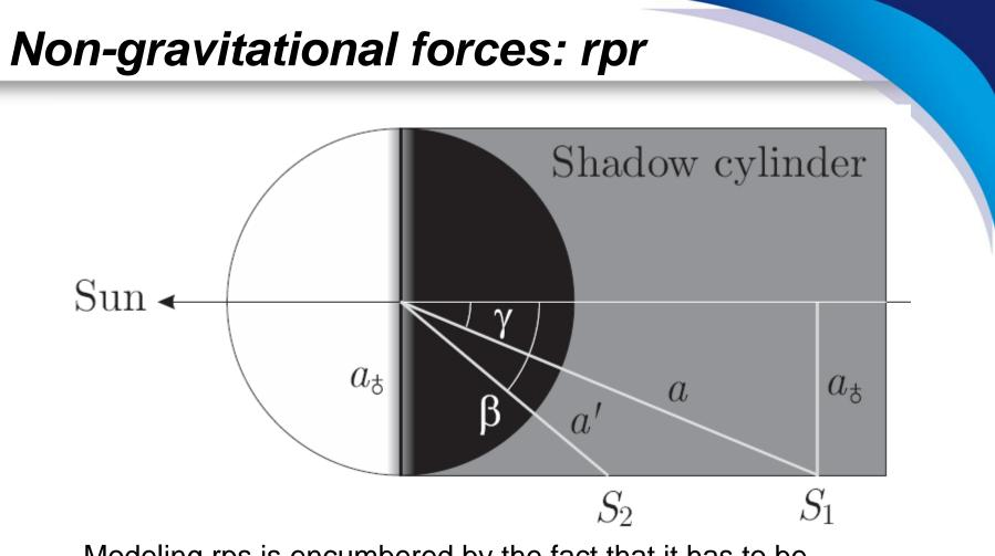
Modeling rps is encumbered by the fact that it has to be switched of, when the satellite enters the Earth's shadow.
