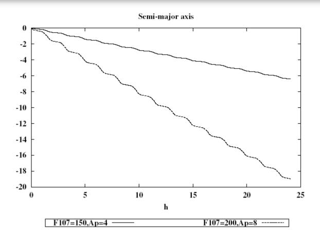
Decay of the sm-axis *a* of GPS/MET making different (but realistic) assumptions concerning the atmospheric density. Bottom line: The sm-axix decreases by several m/day.
