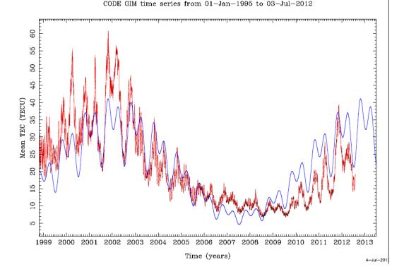
Mean electron content in the upper atmosphere as estimated by CODE (Center for Orbit Determination in Europe). Note the length of the most recent solar cycle.
