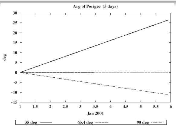
Rotation of perigee distance  $\omega$  for inclinations  $i = 35^{\circ}$ ,  $63.4^{\circ}$ ,  $90^{\circ}$ . For  $i = 63.4^{\circ}$  the perigee stands still. Für  $i < 63.4^{\circ}$  the perigee moves ant-clockwise, for  $i > 63.4^{\circ}$  clockwise.
