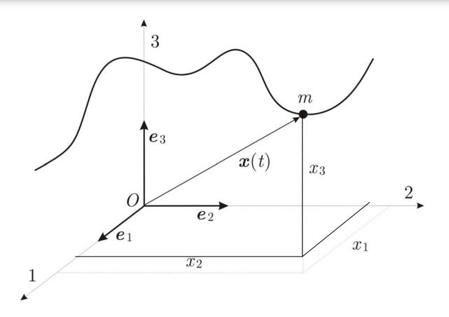
The trajectory of the point mass m is known, if its position vector  $\mathbf{x}(t)$  is known in the IS as a function of time t.
