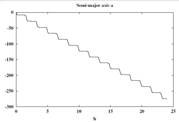
With an eccentricity of e=0.05 instead of e=0.02, the satellity would have penetrated more deeply into the atmosphere and the perturbation would have been much stronger!
