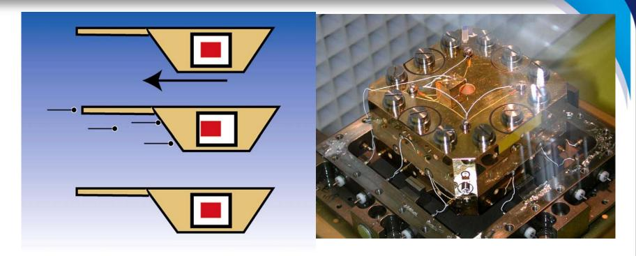
Left: Principles of satellite accelerometry. The motion of a test mass in the shielded interior interior is measured (kept in place through electrostatic forces). Right: real satellite accelerometer..
