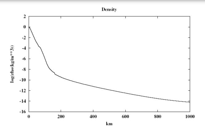
Mean atmospheric density from the MSIS-model. Drag may be neglected above a height of about *2000* km.
