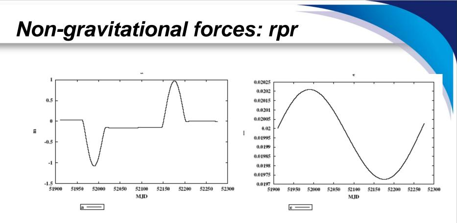
Impact of *rpr* on the sm-axis *a* and on the eccentricity *e* of a GPS-satellite (over the period of one year).
