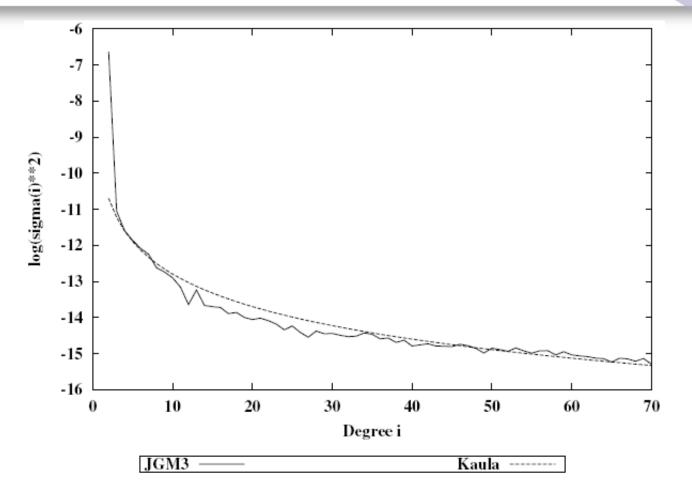
Kaula's "rule of thumb" and the "true" degree amplitudes of degree *i* of the *JGM3*.
