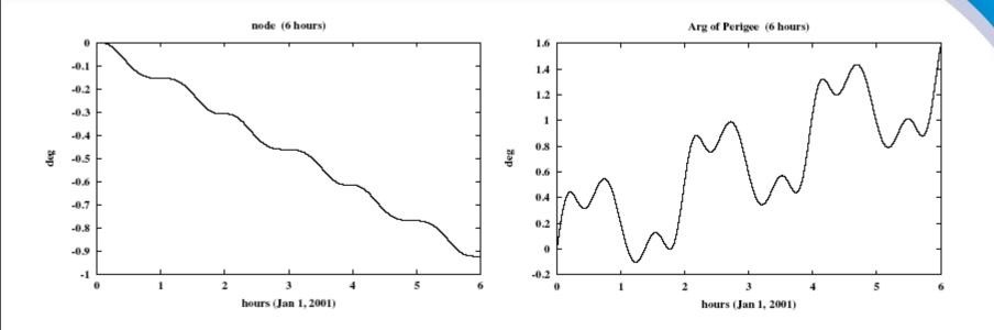
The perturbations in the R.A. of the ascending node  $\Omega$  and in the argument  $\omega$  of perigee also show secular perturbations (the node rotates clockwise, the perigee ant-clockwise – for the initial conditions used).
