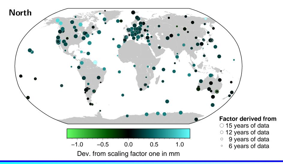
Estimated scaling factors for the atmospheric loading model Deviation from one over 15 years, norm. with the RMS
