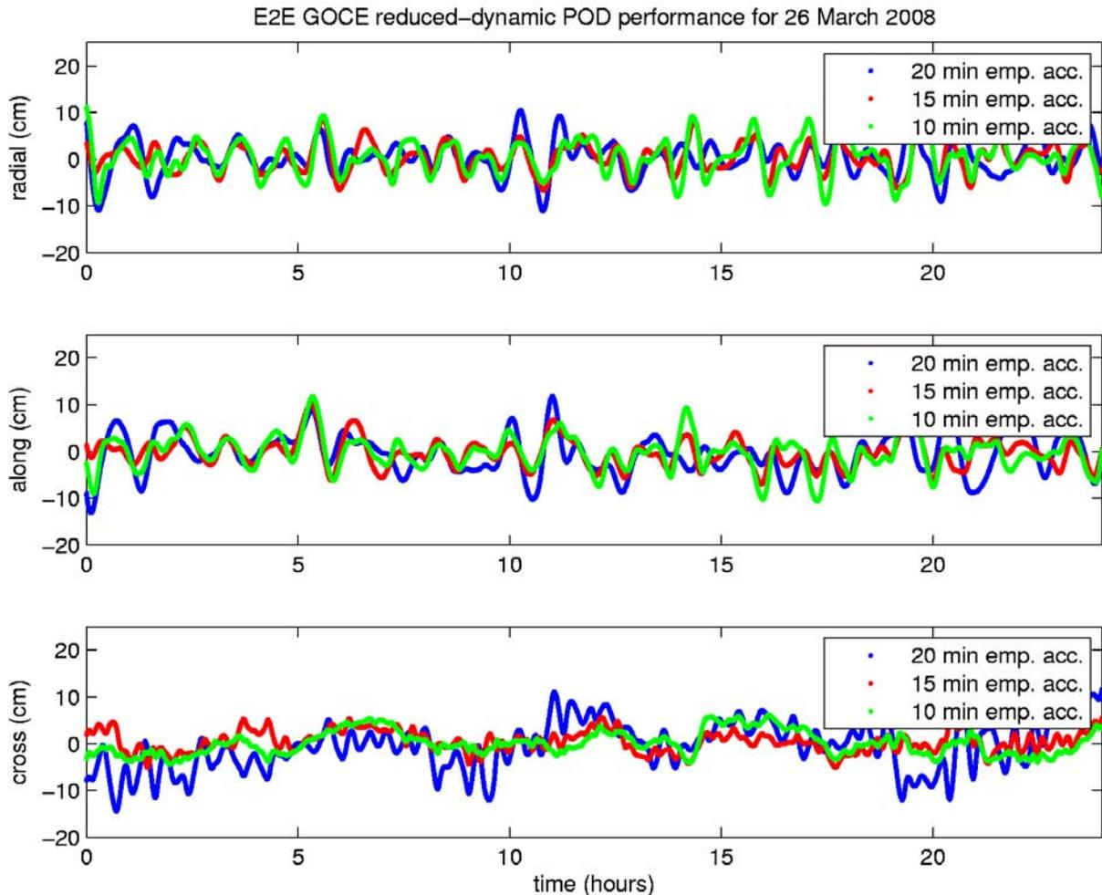
Figure 2. GOCE orbit errors for reduced-dynamic orbit computation with GEODYN using simulated E2E SSTI data for 3 different time intervals for the estimated empirical accelerations
