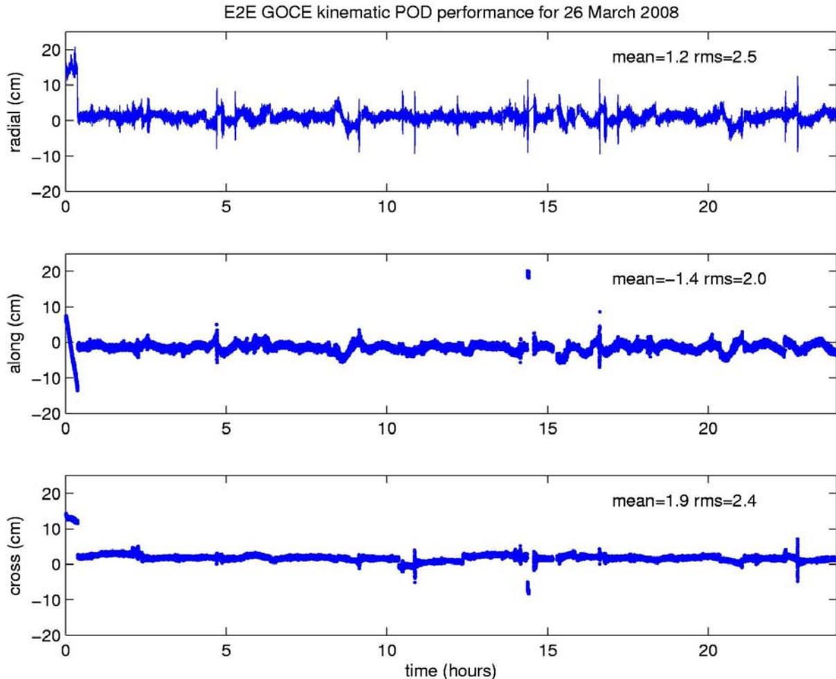
Figure 3. GOCE orbit errors for kinematic orbit computation with GHOST using simulated E2E SSTI data
