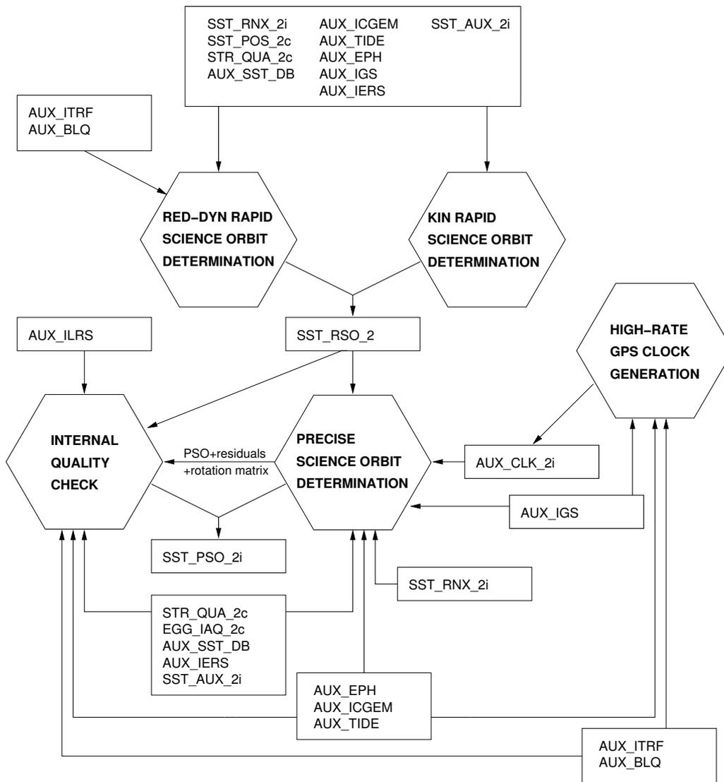
Figure 1. GOCE Precise Orbit Determination architecture (High-level Processing Facility): indicated are the five main modules and several input/output products and data streams.
